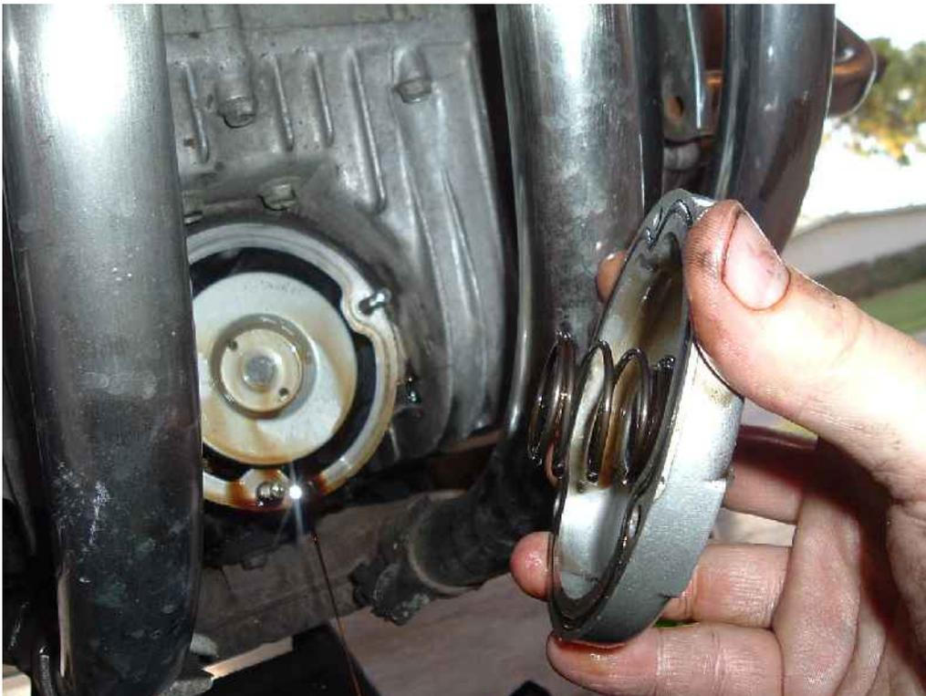
If necessary, use some kind of small sharp object to remove the old O-ring.
