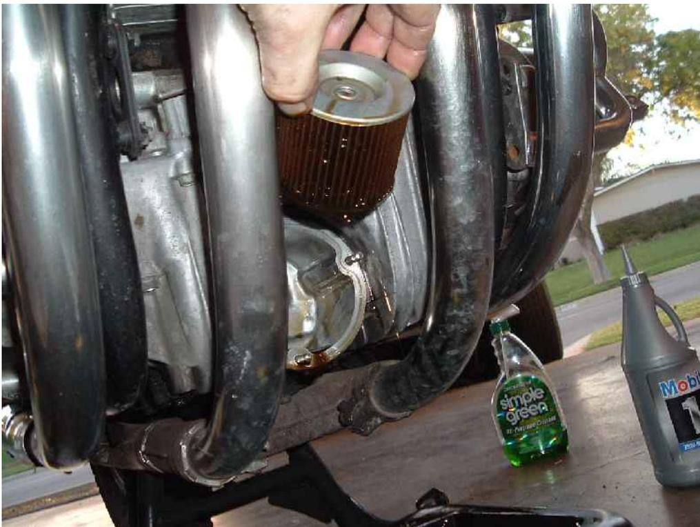
Here is a shot of the empty oil filter cavity. I usually stick my finger in there to rake out the remaining oil.
