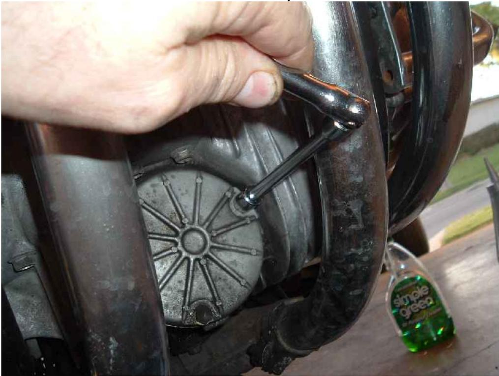
As you are removing the bolts, use your fingers for those final couple of turns so that you can catch the bolts and washers and keep them from falling into your dirty oil. Here the cover is off.
