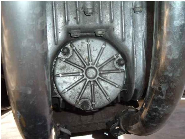
These three "acorn" nuts are 12mm. The cover is also spring-loaded.
