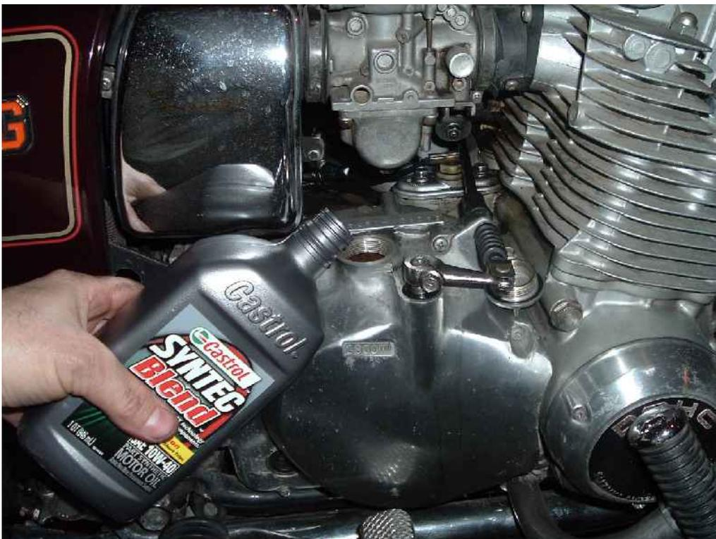
Fill with the recommended amount of oil then check the sight glass located on the right case next to the brake pedal and foot peg.
