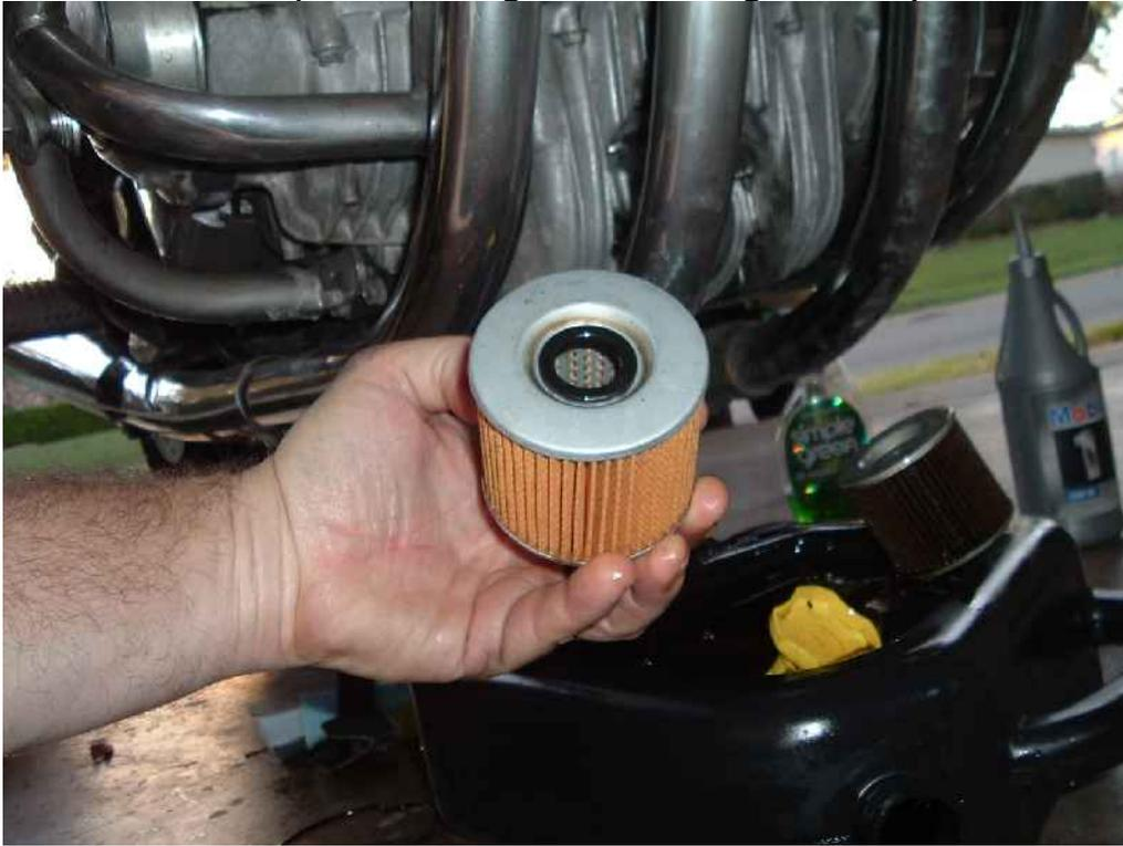
Then just push it back on the center pipe in the filter cavity. Give it a little twist back and forth and make sure it is pushed in all the way.
