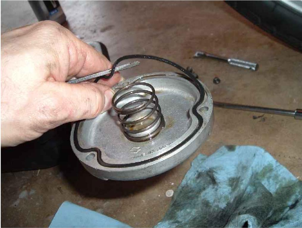
I usually take a shop rag and clean the O-ring channel too. Make sure there is no debris where the O-ring sits on the cover. Now pull out the old filter and let it drain.
