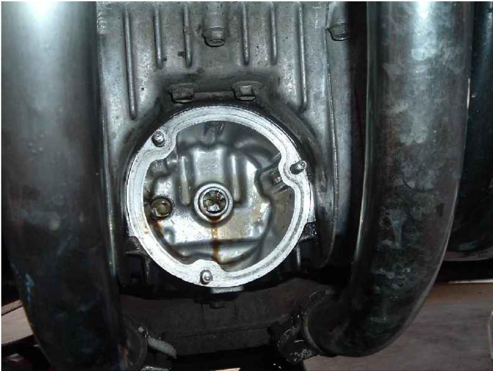
Here we have the new oil filter and O-ring. The next time I change oil I will put the O-ring in a small book for a day or two so that it lays flat. After being scrunched in the box with the filter it doesn't lay well in the cover.
