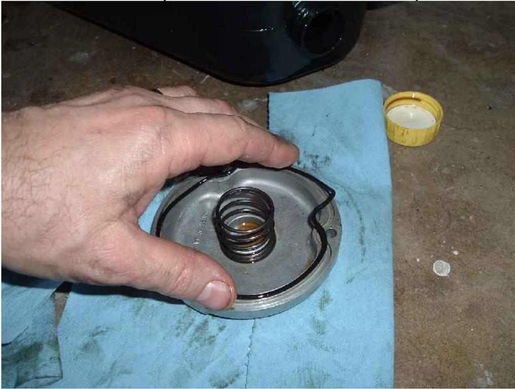
You must hold pressure on the cover while putting the nuts back on. With one hand, tighten them up as snug as you can with your fingers while still holding pressure on the cover with your other hand.
