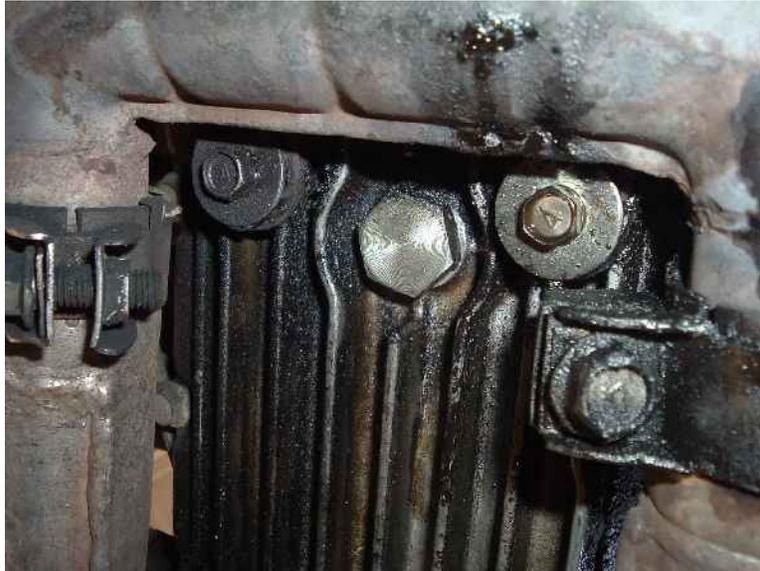
This bolt is the same size as my spark plugs, 21mm if I remember correctly. Put your oil receptacle under this drain plug before you loosen it. Use your spark plug socket or a socket with a short extension to remove the bolt as such:
