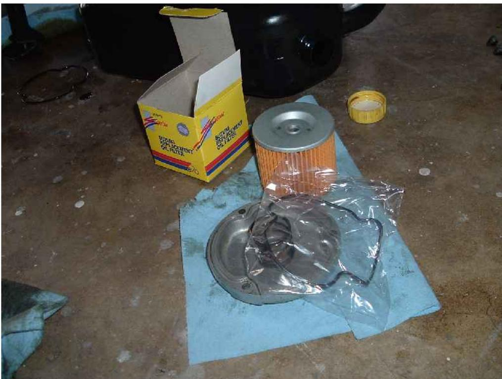
Before I place the new filter back in the cavity I like to rub some oil on the rubber seal. This will help make a good seal right away.
