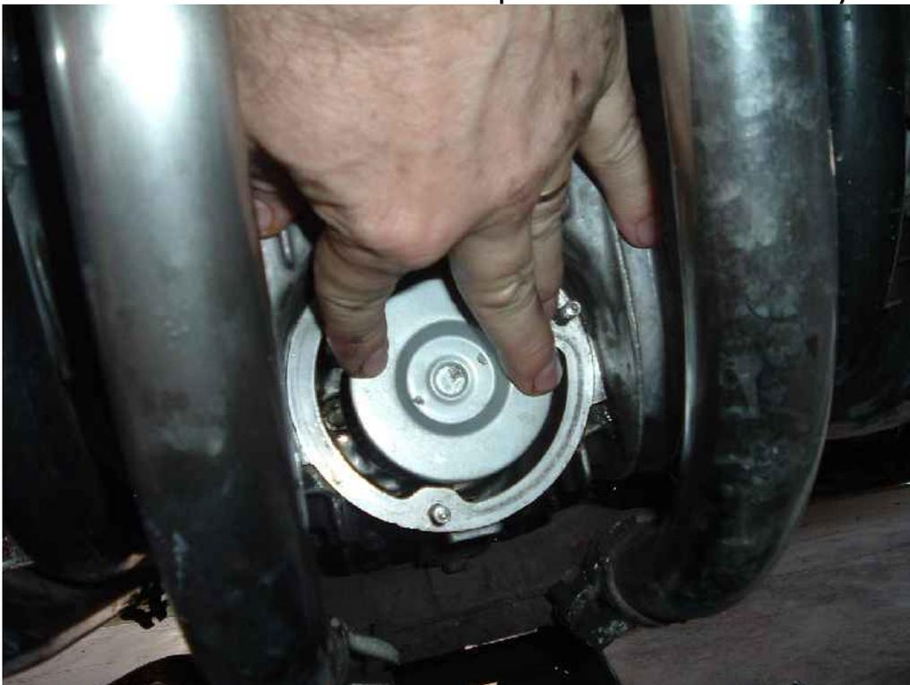
Now place the new O-ring in the channel of the filter cover. If it won't lay down, use some oil or a little grease to hold it in place. You don't want it to come out of the channel as you bolt the cover back in place.
